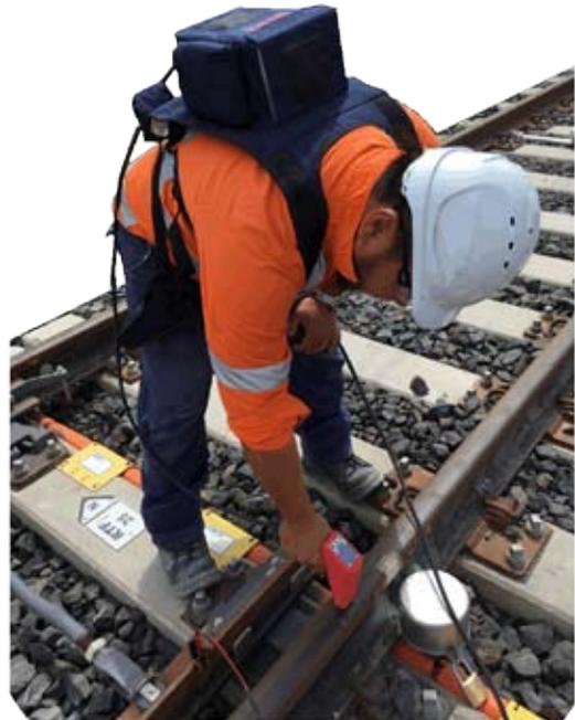
The ECT-4 comes with a 10m and 100m extension cable allowing the operator to probe multiple test points around the earthed or grounded system. Test length extensions may be ordered in multiples of 100m.
